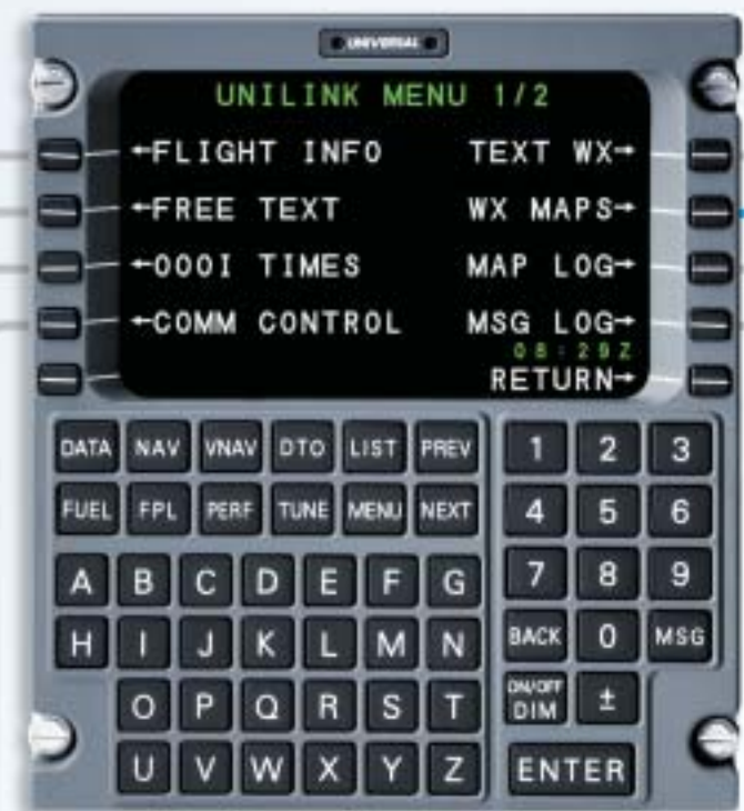
UNS Flight Management Systems can provide control and display for UniLink features and capabilities.
